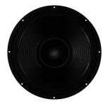
This next evolution subwoofer uses a new, longer, four layer aluminum voice coil. The result is more energy in the gap, less heat, higher sensitivity, higher power handling, lower distortion and better overall performance. The 18DS115 features a 40mm long, 4.5 inch diameter (116mm) Copper Clad Aluminum Wire voice coil. With a 1700watt AES power rating, 98 dB sensitivity, and over 14.0mm of Xvar, this high energy subwoofer is a significant step forward from similar models in the B&C range.
