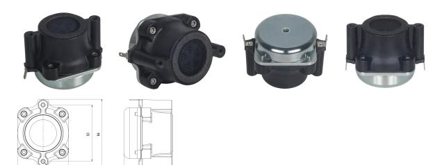
Ultra Compact 48mm diameter 40 W continuous program power capacity 1" horn throat diameter 36 mm (1.4 in) aluminium voice coil HT Polymer diaphragm 1000 - 17000 Hz response 108 dB sensitivity
